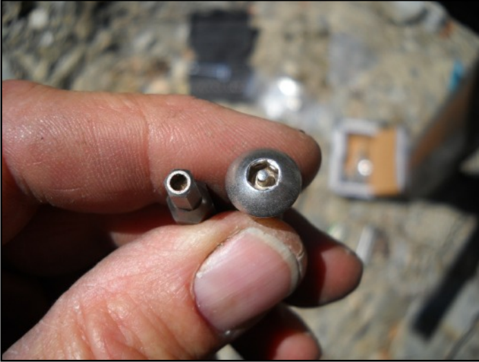
Theft-resistant security bolt, requiring a specialized driver to install.
