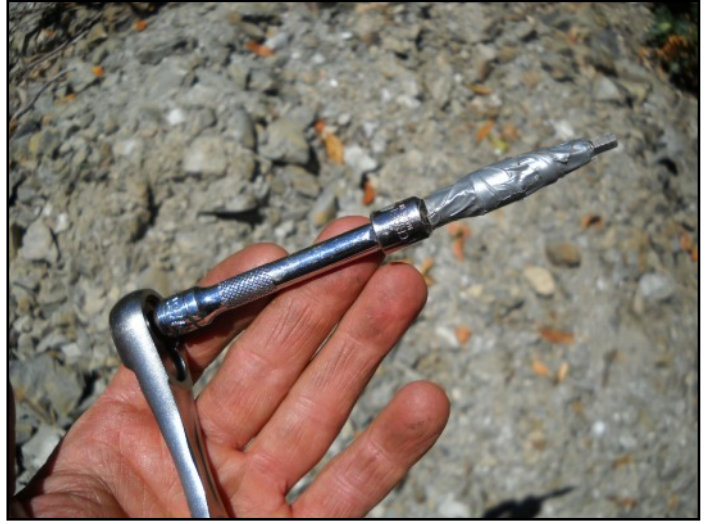
Wrap tape around the wrench and Torx bit to avoid losing it.
