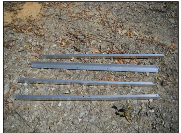
These are the ribs that hold up the solar panels.
