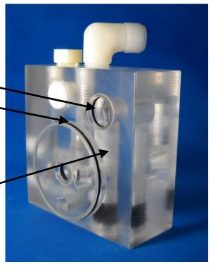
Leaks around the Slotted Plugs cause pressure loss. Replace the teflon tape or install a new Slotted Plug 1/4", 10-1387
