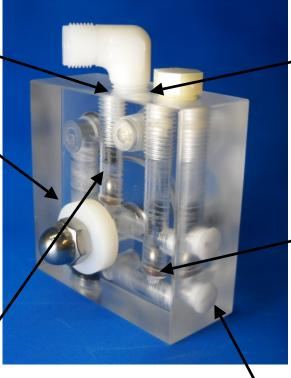
A crack in the clear plastic between the fittings will cause a serious leak. Sometimes it can be sealed with Crazy Glue, but usually the Head has to be replaced.
