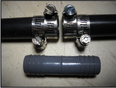
Use four clamps on connectors
