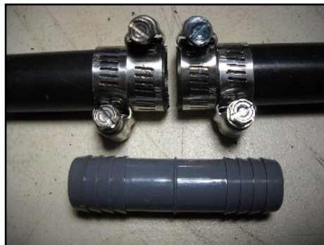
Join pipe pieces with four clamps. For details on working with poly pipe, see "Input and Output Pipe Details" in the High Lifter section.
