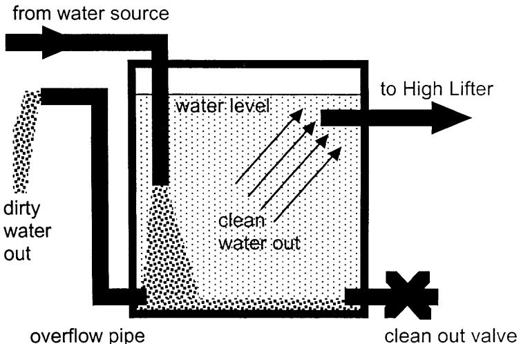
A 300 gallon tank works great, but even a 55 gallon drum is better than nothing. Sand getting into the pump can wear it out in a year.
