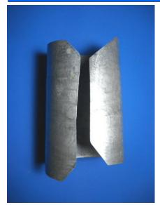
Low Pressure Piston and Collar Installation Tool. Make the tool from aluminum roof flashing, which can be obtained at hardware stores. Cut out a piece measuring 5" x 7.5". Trim the corners and sand down sharp edges. Form it into a round shape.
