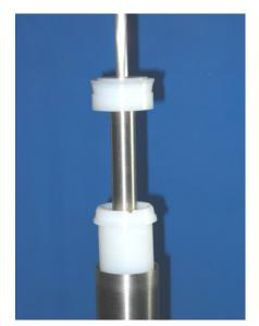
Slide the lower edge of the Collar into the Installation Tool.
