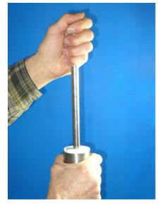
The second Low Pressure Piston can be slid into the Barrel without using the Installation Tool because its lip is oriented away from the Barrel.
