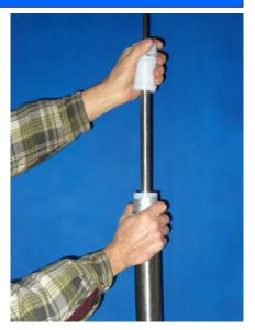
Insert the High Pressure Cylinder Assembly into the Barrel. Then slide the lip of the first Low Pressure Piston into the Installation Tool. Push on the Assembly to make it slide into the Barrel.
