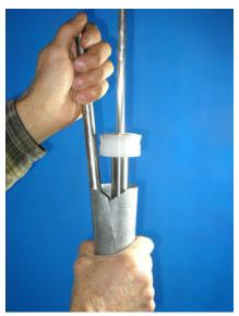
Push on the Collar with a rod such as the Comm Tube. This is how the upper lip of the Collar goes into the Barrel. Otherwise the upper lip would catch on the edge of the Barrel.
