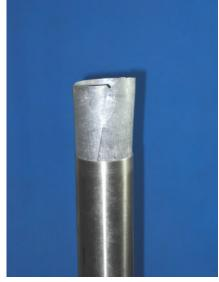
Insert the Installation Tool into the Barrel.
