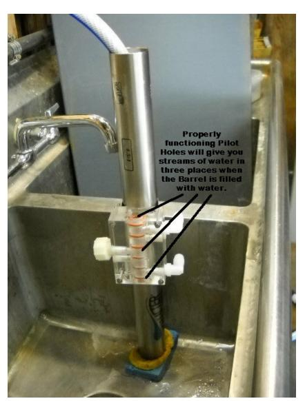
Usually the center Pilot Hole gets clogged. You can see if one of these is clogged by disassembling the HL, upending it in a sink, and filling it with water. Turn the flow from the hose down to a trickle so it doesn't overflow the barrel. You should see a stream of water ejecting from three locations inside the Valve Body.
