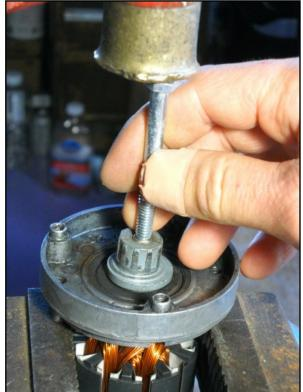
This Drive Cam is in good shape. If the ridges of your Drive Cam are worn off, it can slip in the pump head and cause loss of power to the pump head.
